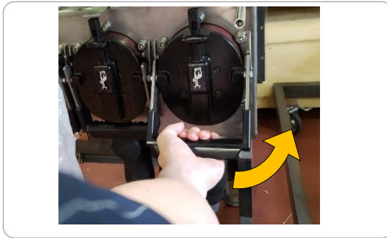
Figure 38. Lever operation (⑧)
